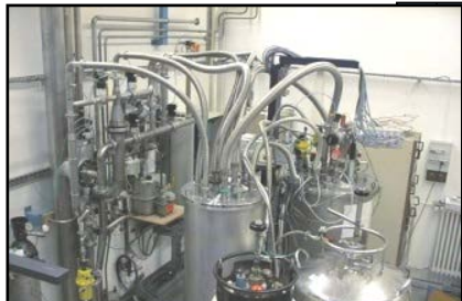
LHC : Calibration of all Cernox thermal sensors (> 6000 units)
