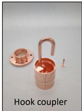
3D-printed prototype (Epoxy Accura 48) copper-coated @CERN
