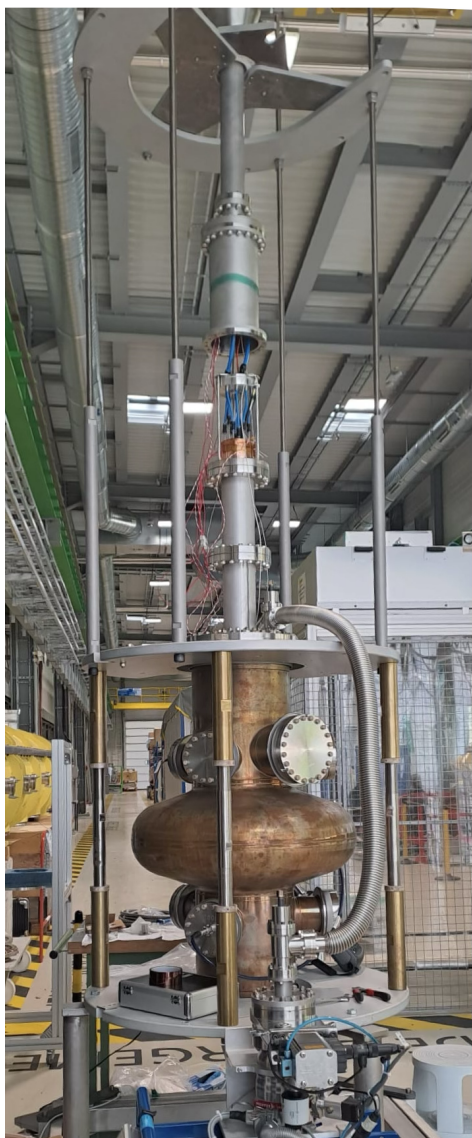
Figure 10: Tuner and transmission line connected to warm 400 MHz LHC cavity.
