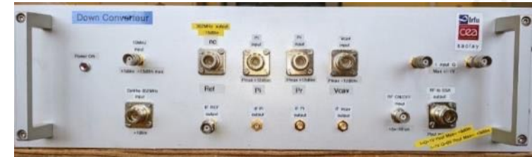
RF interface (frequency translation to 10 MHz)
