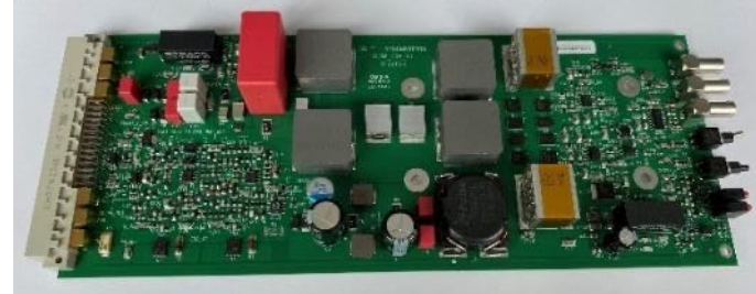
Power converter cards
