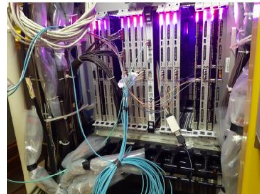
LHCb ECAL upgraded electronics
