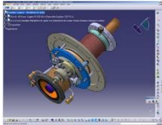
RF Coupling ESS project
