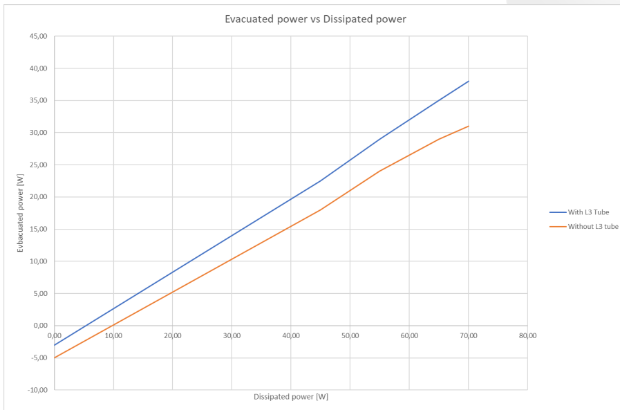
Evacuated power vs Dissipated power
