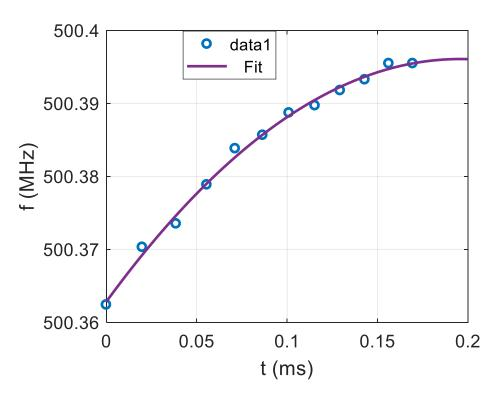
Result of screenshot processing. Bunch circulating frequency vs time.
