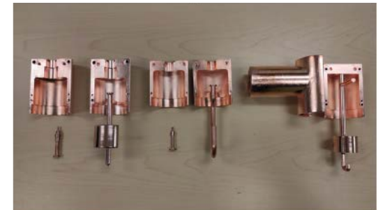
Probe, Hook and DQW HOM couplers for PERLE (from left to right) C.Barbagallo et al, IPAC2023
