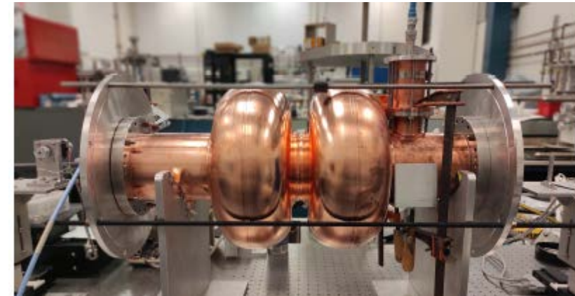
First RF measurements of coaxial HOM prototypes for PERLE C.Barbagallo et al,IPAC2023.
