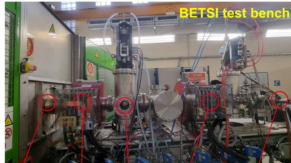
Source exit      Solénoïd 1      Diagnostic location (WF or EMU)      Solénoïd 2      Cooled beam dump with current measurement
