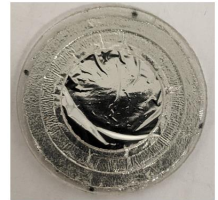
Figure B.5: Front and backside of a ^{114m}\text{In} source prepared at KU Leuven.
