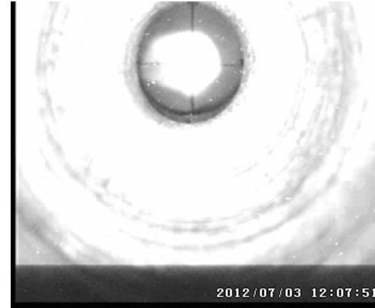
Optimized electron beam sizes at the exit of linear accelerator (RMS sizes: x-direction is about 5 mm, RMS sizes: z-direction is about 5 mm,)
