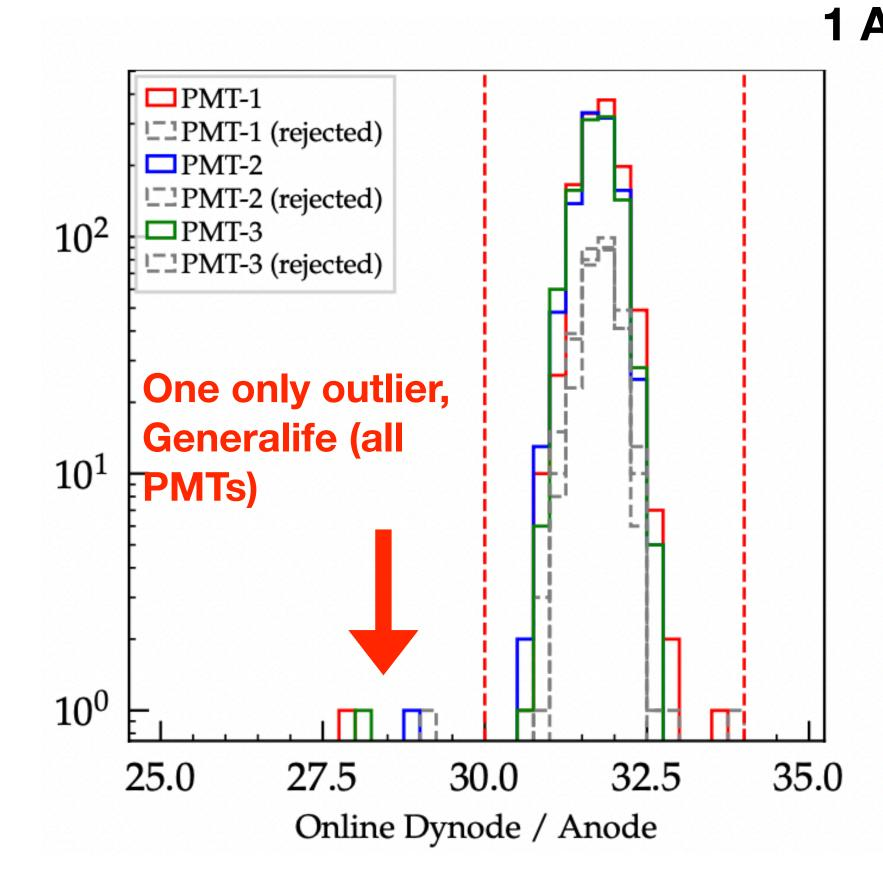
**Proposal to set tolerances at 29 < HG/LG < 33 to alert on outliers that may indicate failures**
