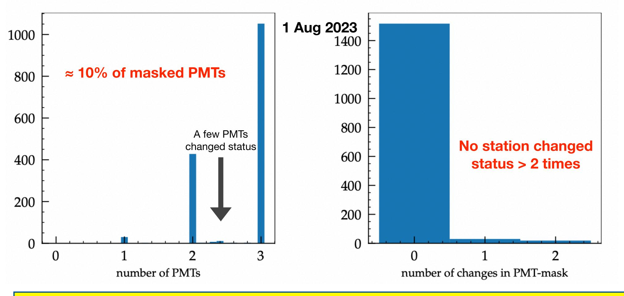
**Proposal of an alert/quality selection based on the mask parameter (station**level) : same cut as used for the UB, i.e., more than 2 changes per day.
