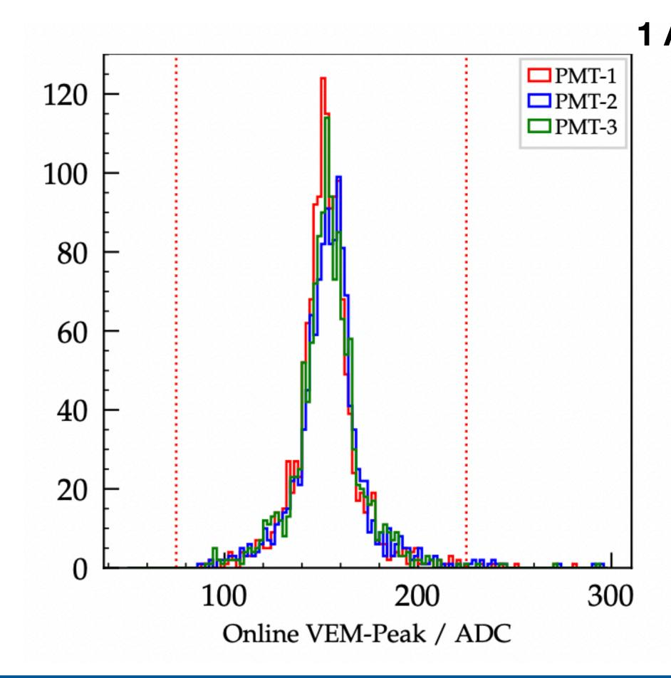
**Proposal to set an anomaly-alert at Mean(VEM-Peak) < 50 ADC and <Mean(VEM-Peak) > 300 ADC.** And an instability-alert at  $\sigma_{VEM-Peak} > 2.5$  ADC
