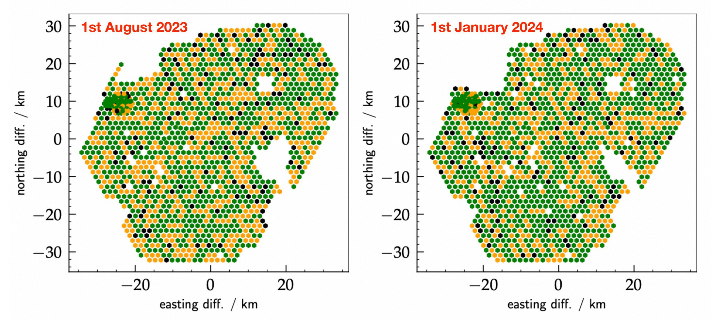
The so-called Martin's Maps: daily "commissioning" of the UUB-SD after applying selections based on monitoring-data studies. Green: stations with all PMTs/channels OK; Orange:  $\geq 1$  PMT/channel non OK; Black: non-OK stations
