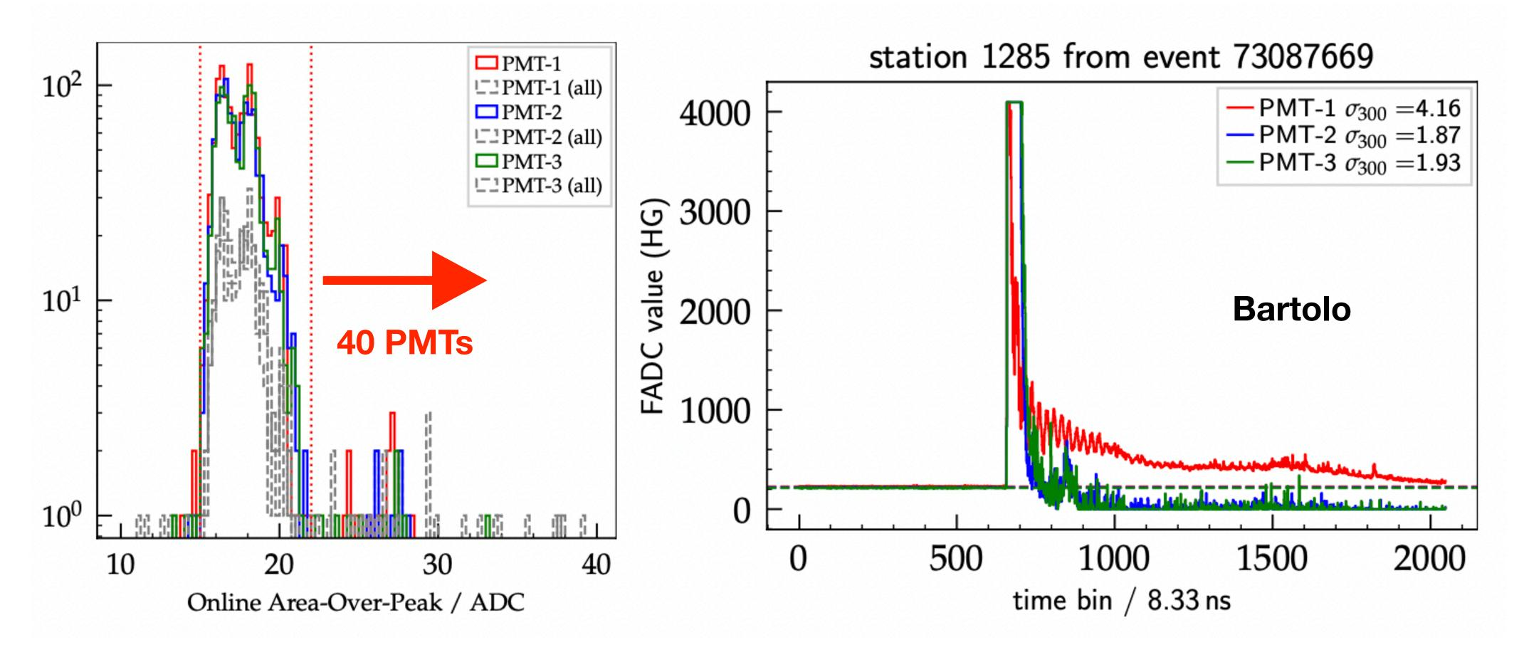
**Proposal to set an alert on the current "pseudo" AoP if the value is outside the tolerances 15 < AoP < 22 N.B.** Tolerances to be revised once the calculation of the VEM charge is updated
