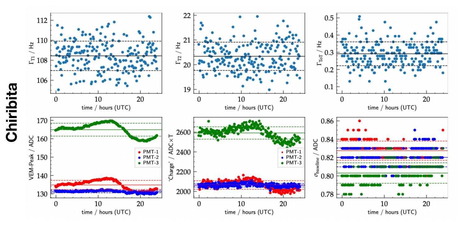
To get a list with a higher "purity" of truly problematic PMTs, the tolerance on  $\sigma_{VEM-Peak}$  may be obviously changed (at the risk of non-identifying true bad-PMTs) A study on temperature dependence of the VEM peak is recommended
