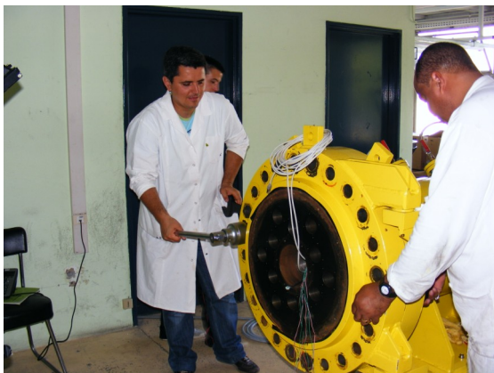
Figure 3: Closing the pressure vessel before a test.
