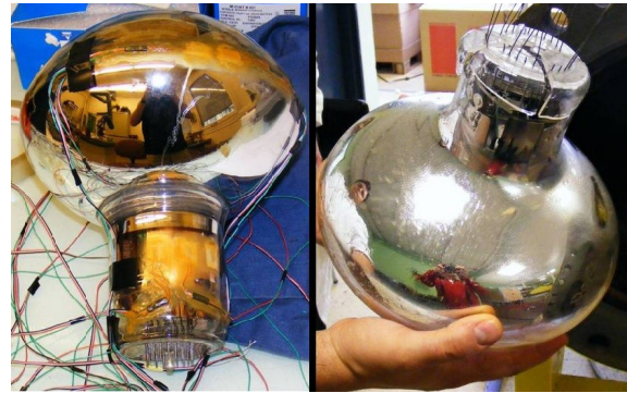
Figure 4: Left: PMT equipped with stress gauges. Right: PMT cracked after a pressure test.
