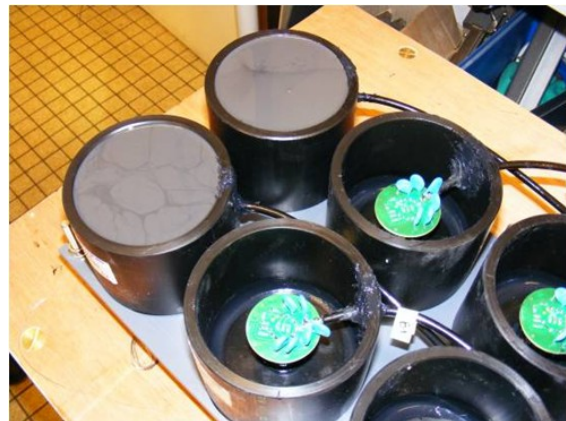
Figure 2: Potting of 1-in PMTs. The PMT base can be seen on the right side of the picture. The potted circuits are on the left side.
