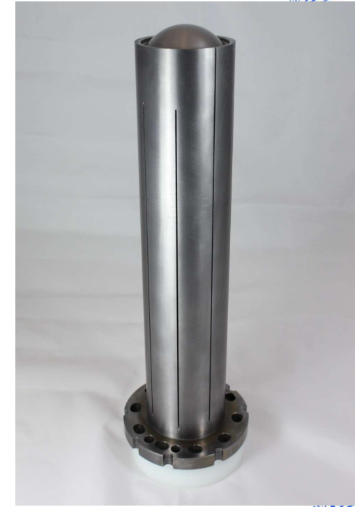
Final Assembly (ALL COMPONENTS FITTED AND THERMOCOUPLE GROVES MACHINED)
