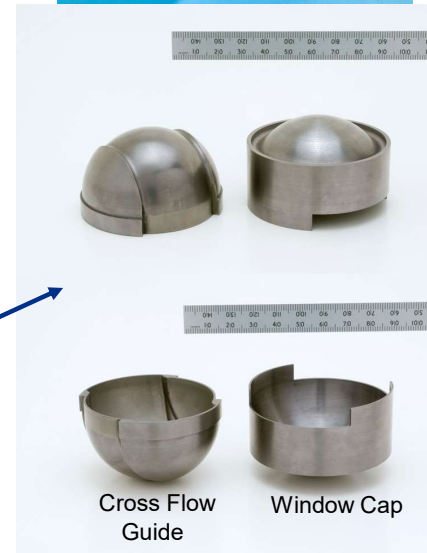
Machined from solid Ta rod
