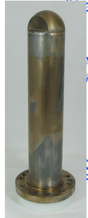
EB Welded + HIP 1250 °C 1400 MPa
