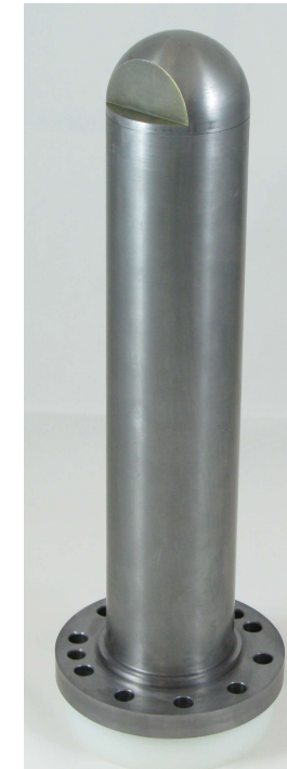
Ta Flange + W Core + Ta Tube + Ta Cap
