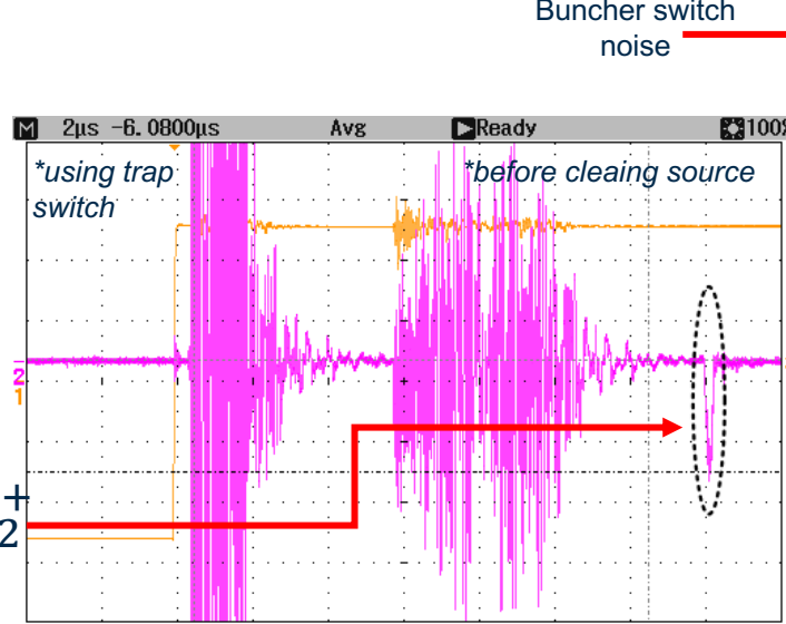
Signal on MCP for one revolution, \text{ToF} = 13,69\mu\text{s} .
