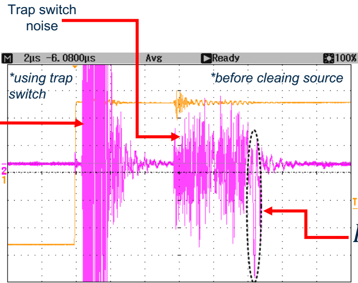
Signal on MCP for a shoot through, \text{ToF} = 10,85\mu\text{s} .
