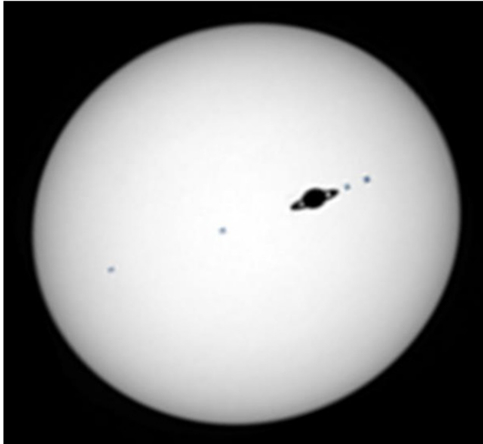
Figure 11. A vision of microarcsecond optical imaging: Expected resolution for an assumed transit of a hypothetical exoplanet across the disk of Sirius, using the Cherenkov Telescope Array as an intensity interferometer. Stellar diameter = 1.7 solar, Distance = 2.6 pc, Angular diameter = 6 mas; assumed planet of Jupiter size and oblateness; Saturn-type rings; four Earth-size moons; equatorial diameter = 350 \mu as. With the CTA array spanning 2 km, a 50 \mu as resolution provides more than 100 pixels across the stellar diameter.
