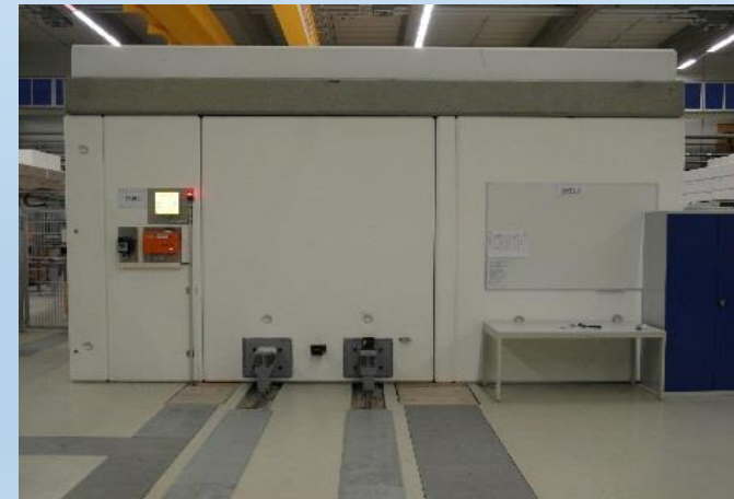
Cryomodule test stand – front view
