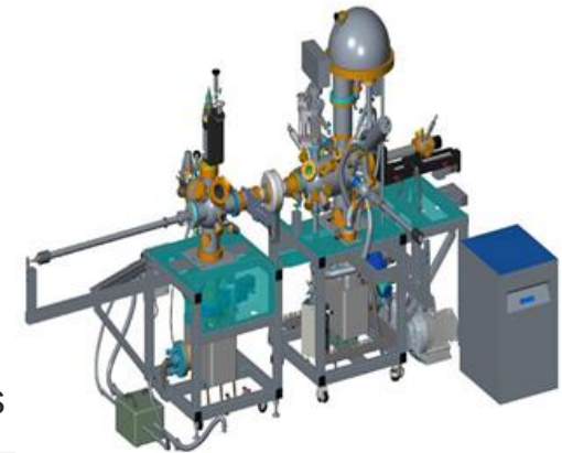
SEY measurement set-up at cryogenic temperature @ IJCLab (2024)
