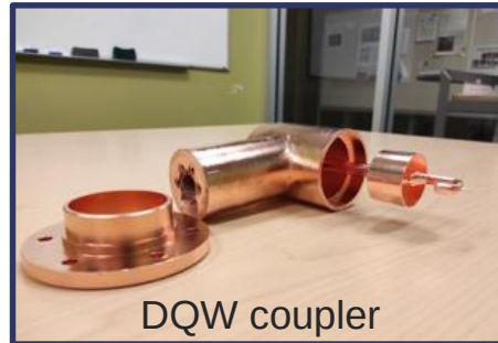
3D-printed prototype (Epoxy Accura 48) copper-coated @CERN
