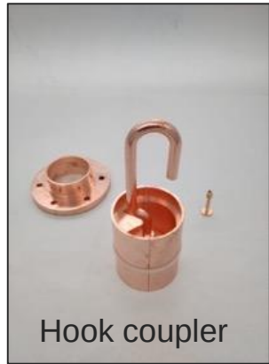
3D-printed prototype (Epoxy Accura 48) copper-coated @CERN
