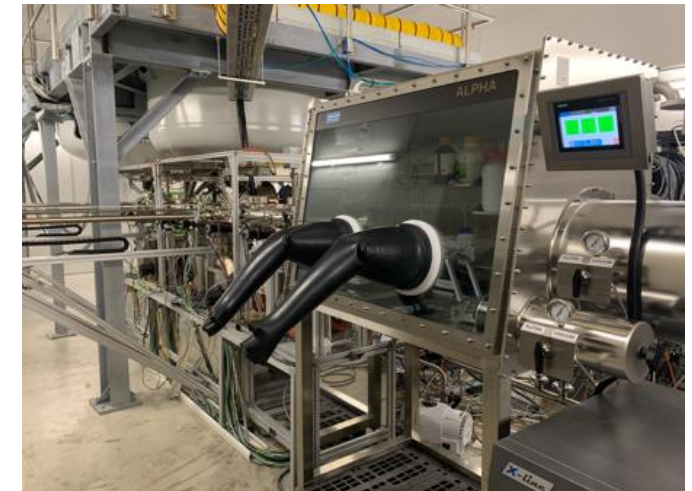
A Photocathode Preparation Facility (PPF)
