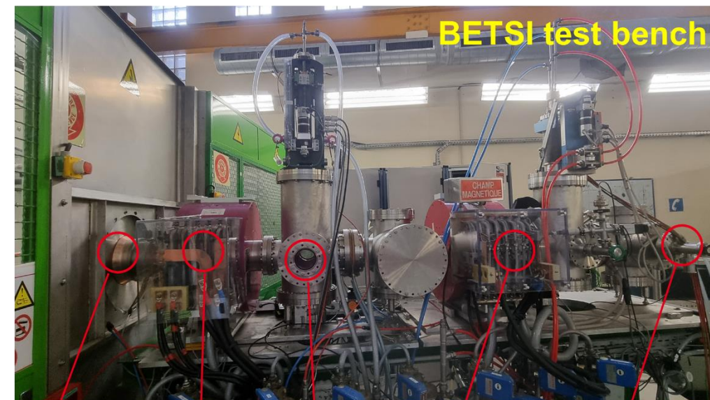
Source exit Solenoid 1 Diagnostic location (WF or EMU) Solenoid 2 Cooled beam dump with current measurement
