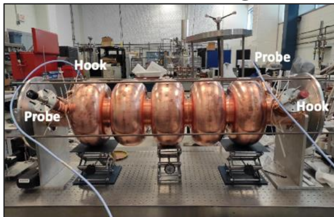
3D-printed prototype (Epoxy Accura 48) copper-coated @CERN
