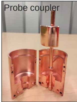
3D-printed prototype (Epoxy Accura 48) copper-coated @CERN
