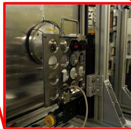
Cell samples/detector holder and robotic arm.
