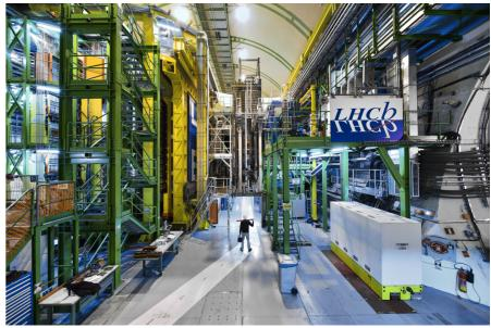
LHCb is a forward spectrometer in the LHC, specialised in the measurements of b- and c-quarks!
