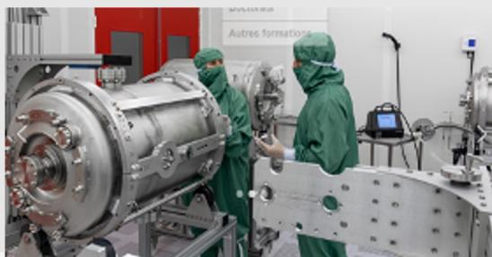
**SUPRATECH** platform dedicated to **R&D on the superconducting cavities** of the future high-energy, high-power particle accelerators. Equipment to prepare, package, assemble and test superconducting RF cavities for IJCLab projects.
