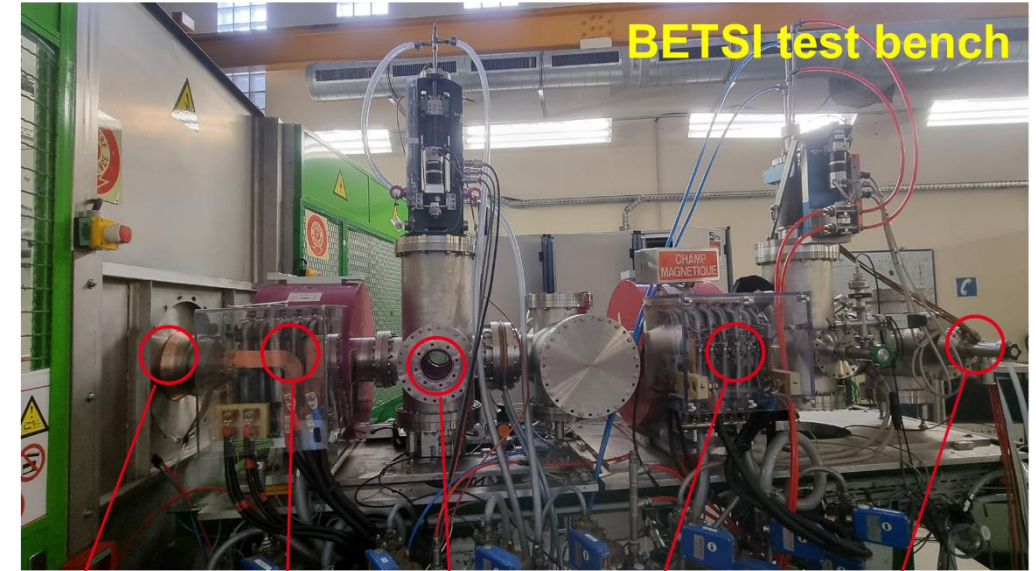
Source exit Solenoid 1 Diagnostic location (WF or EMU) Solenoid 2 Cooled beam dump with current measurement
