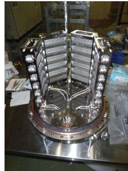
NEG pump set
