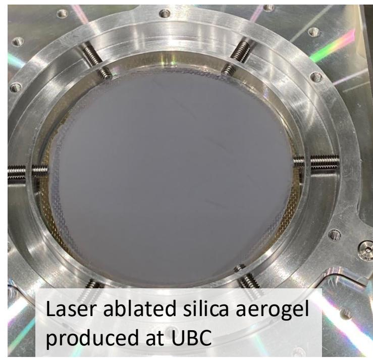
Laser ablated silica aerogel produced at UBC
