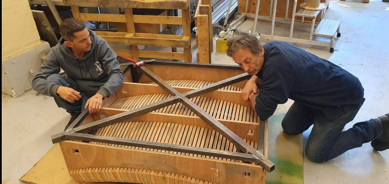
Iron frame to ensure the spherical shape of the permanent magnet support
