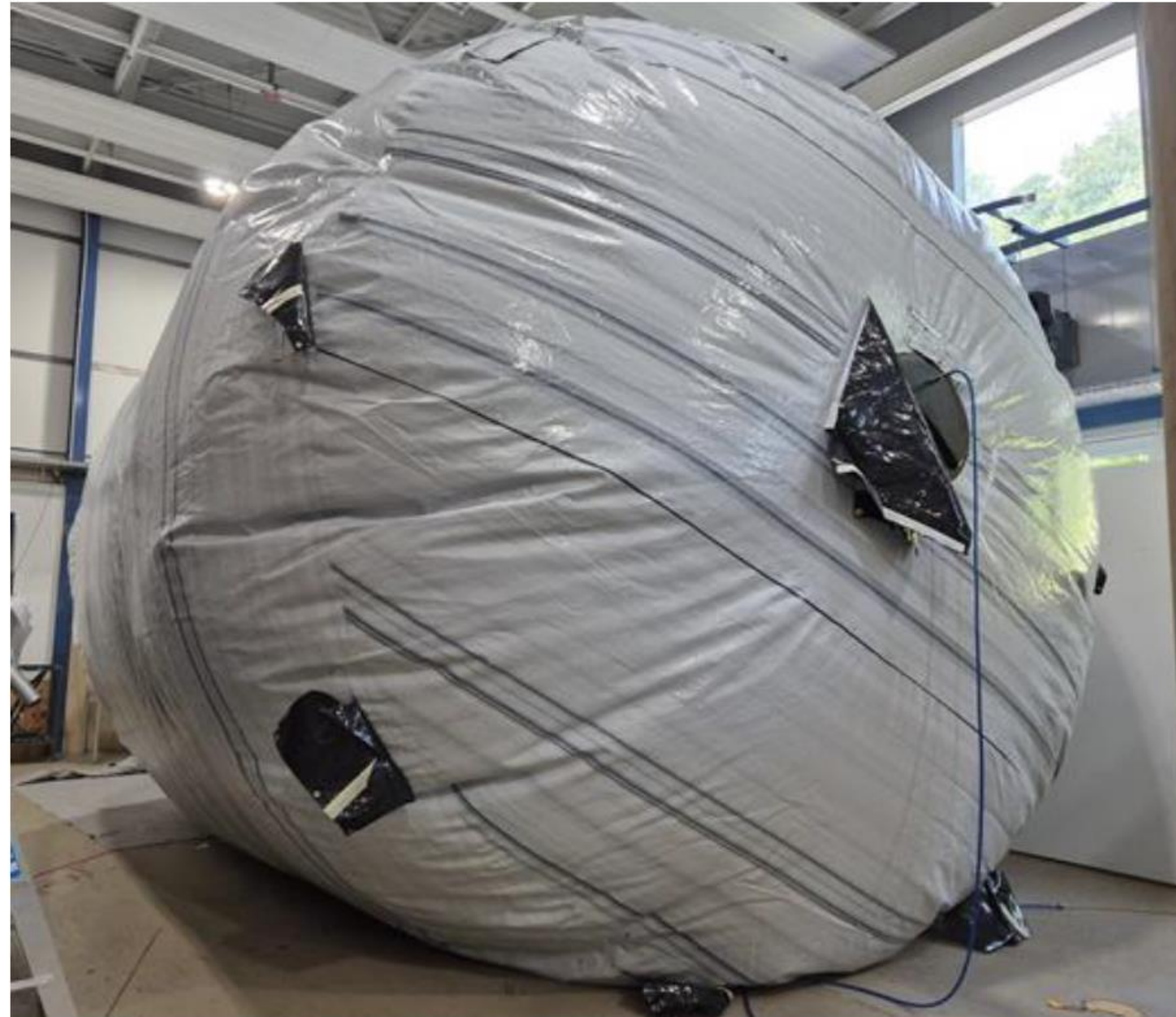
Inflated with air to check for light leaks
