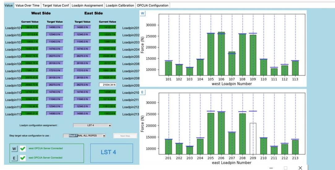
Loadpins Values for Tensionning Telescope Arch
