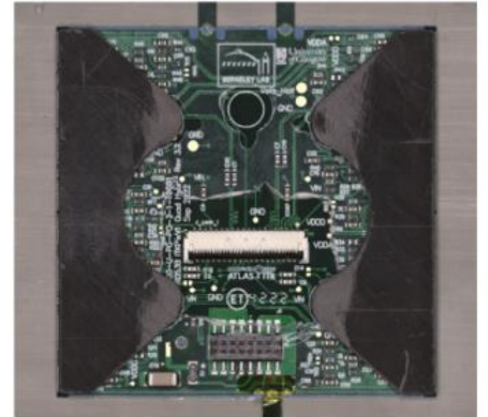
d) Outer Barrel quad module with carbon fibre wire bond protection
