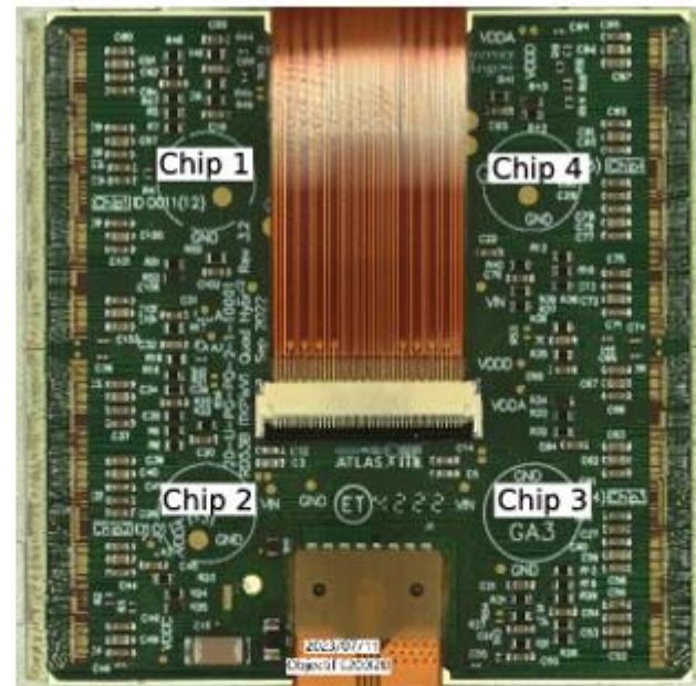
c) Inner System and Outer Endcaps quad module with data and power pigtails connected
