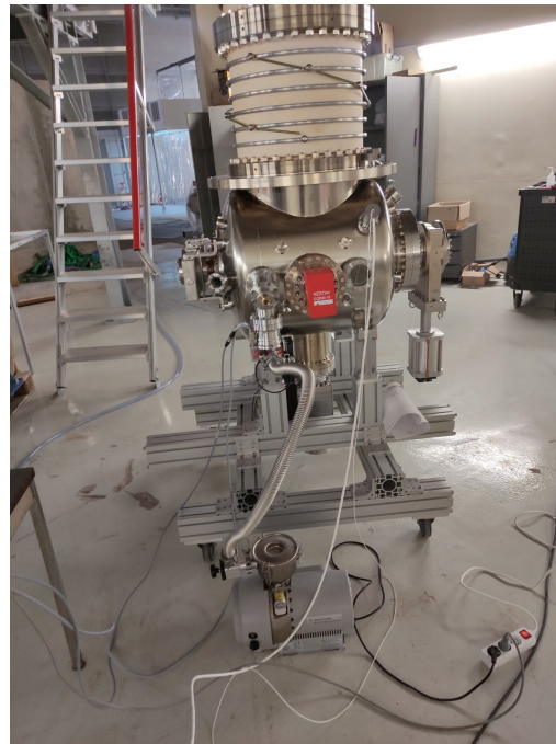
Gun chamber under vacuum (26-05)
