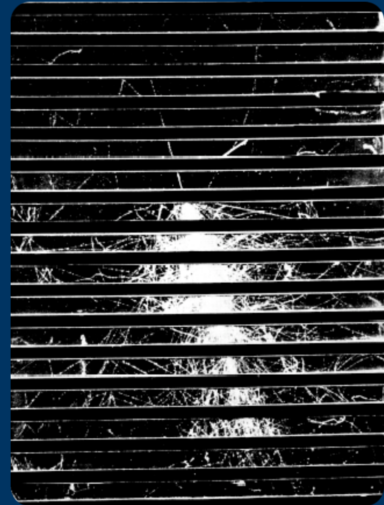
IMAGE OF A SHOWER, AS SEEN IN A CLOUD CHAMBER AT 3027 M ALTITUDE, FRETTER 1949 (PRIMARY PROTON OF \approx 10^{10} EV)
