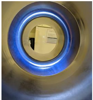
Blueish surface observed on ESS geometry 1Cell cavity
