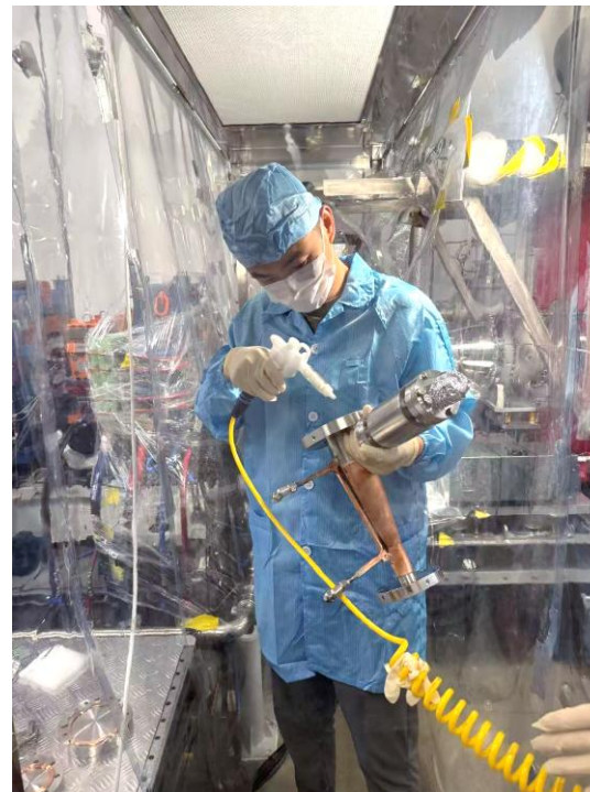
Purge w/ dust-free nitrogen
