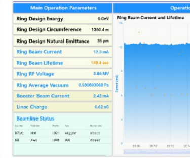
Aug. 18, 2024 Electron beams with currents higher than 10mA were successfully stored.
