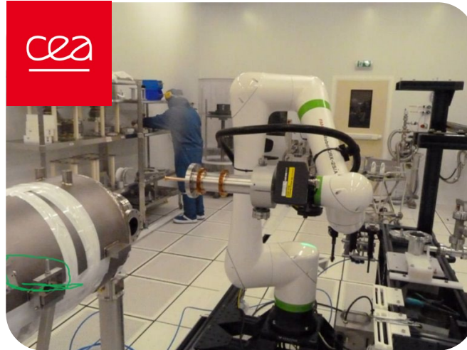
HPC installed with robotic tool
