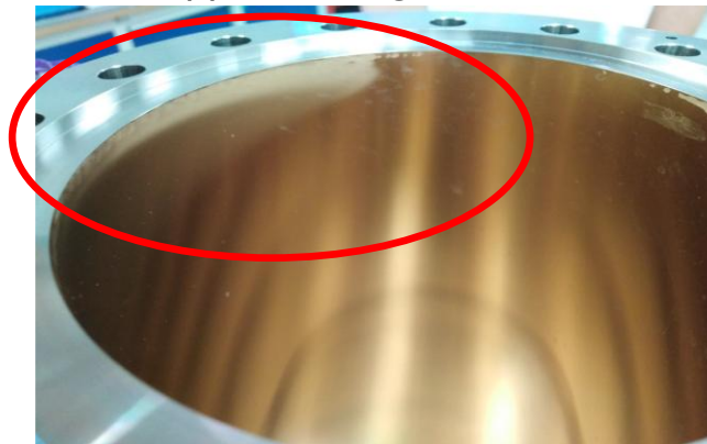
Copper coating with stains
