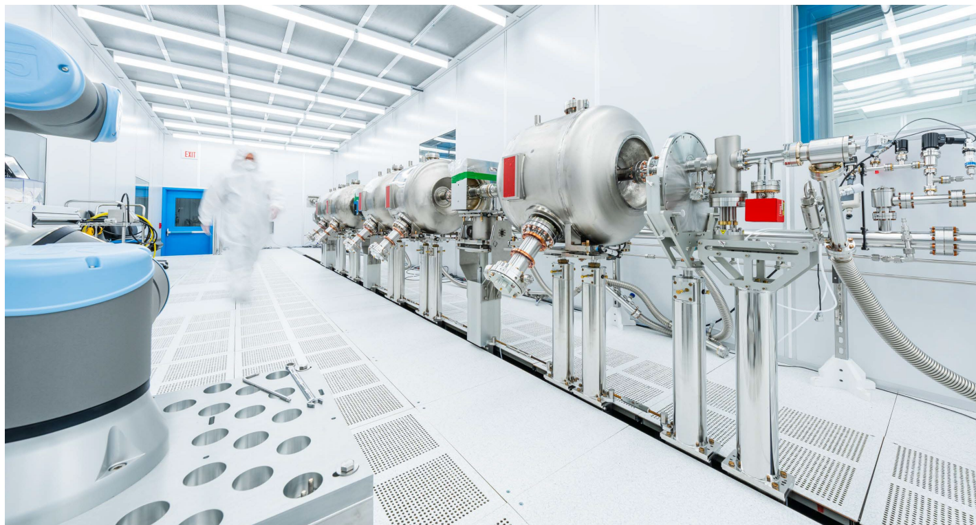
Pre-production SSR2 Cavity and Magnet String Completed using 5 FE Free Cavities
