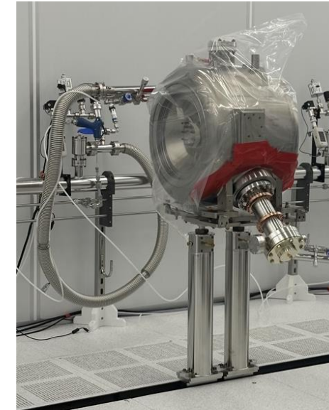
S1-ZA-001 with vacuum side HPC @FNAL after cobotic assembly
