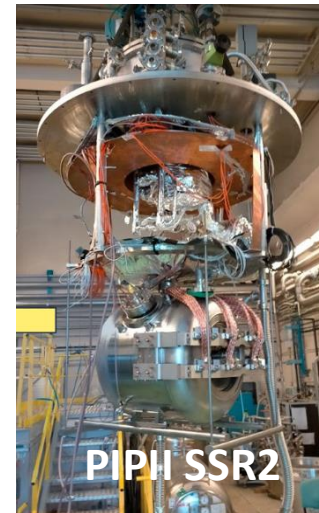
After accidental venting of one spoke module
