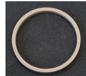
HZB ring after waterjet cutting
