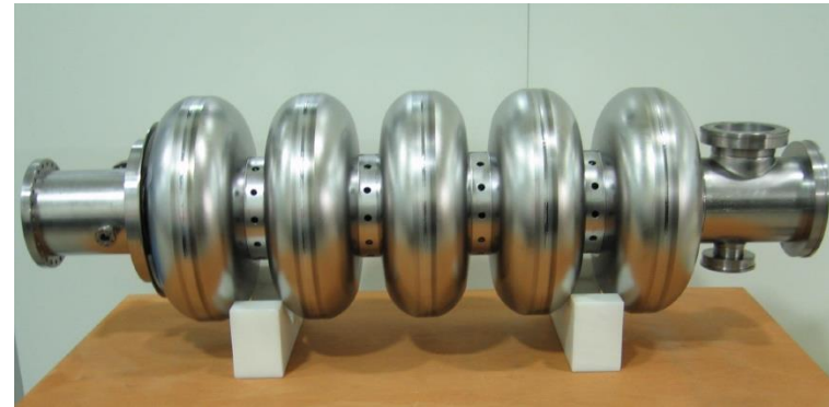
ESS 5-cell cavity, \beta=0.86 , f=704\text{ MHz}
