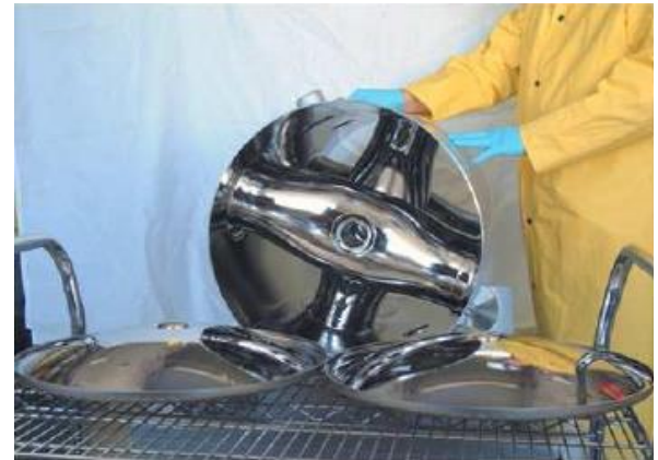
RIA 3-spoke cavity, \beta=0.63 , f=340 MHz
