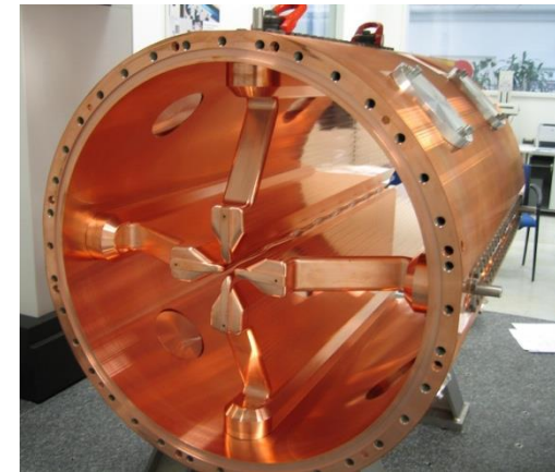
Spiral2 RFQ section, 88 MHz, 240kW 20 keV/u \Rightarrow 0.75 MeV/u, 5 mA
