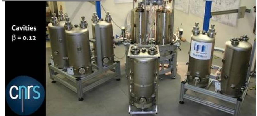
Spiral2 QWR, Nb, \beta = 0.12 , 88 MHz
