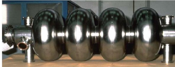
Niobium elliptical cavities: size Vs frequency
