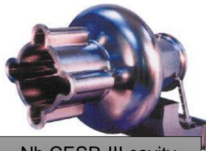
Nb CCSR-III cavity (Cornell), 500 MHz
