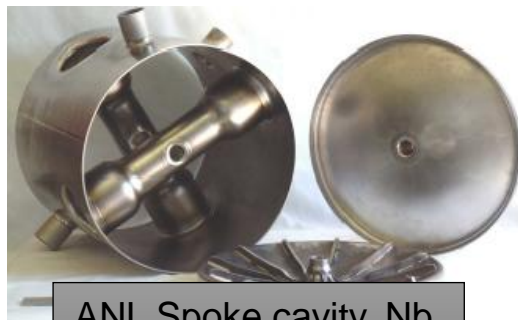
ANL Spoke cavity, Nb, \beta = 0,4 , 345 MHz
