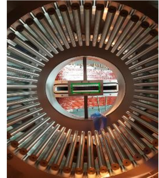
Example of a 48 poles electric multipole
