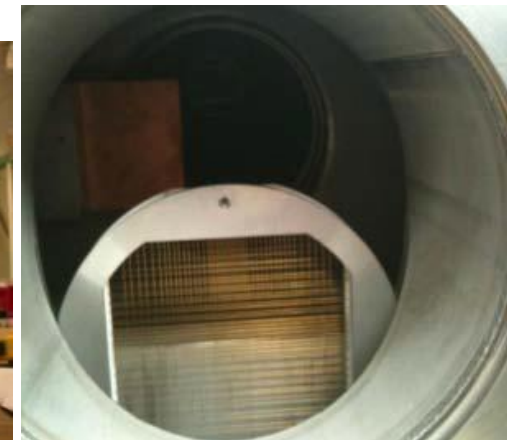
Beam profiler and associated "scraper"
