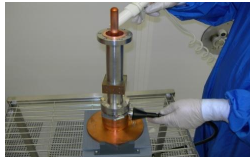
Systematic counting of dusts of the piece mounting on cavities
