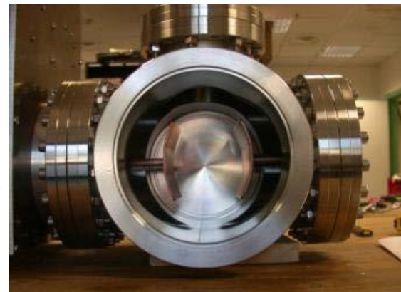
Hacheur (chopper) electrodes
