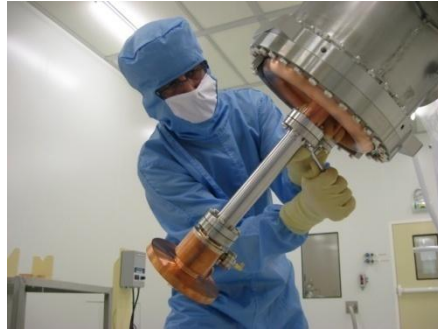
Assembling of coupler on the cavity
