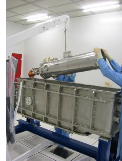
Cavity implantation in the vacuum chamber in the clean room
