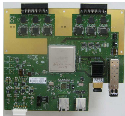
CDC FEE board featured with Xilinx Virtex-5 FPGA
