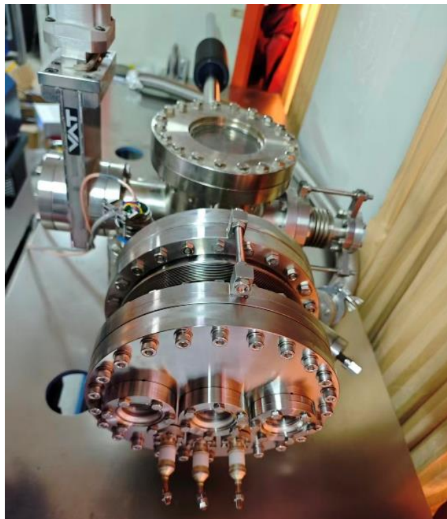
MTE measurement chamber. Left: 3D Model, Right: photograph
