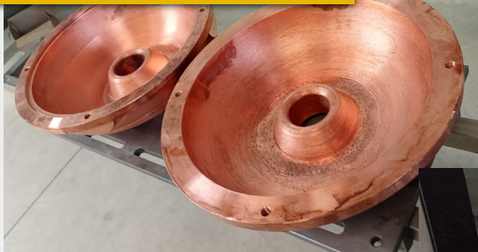
Buncher two halves after machining
