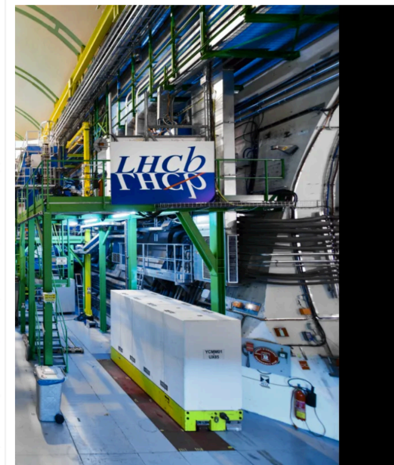
The LHCb detector, at 5600 metric tonnes, is 21 meters long, 10 meters high, and 13 meters wide, optimized for detecting and studying particles (and their subsequent decays) that contain b-quarks inside them. At present, there are over 1500 scientists, engineers, and technicians that work on the LHCb collaboration.
