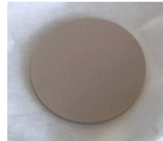
A BST(M) Ferroelectric Sample
