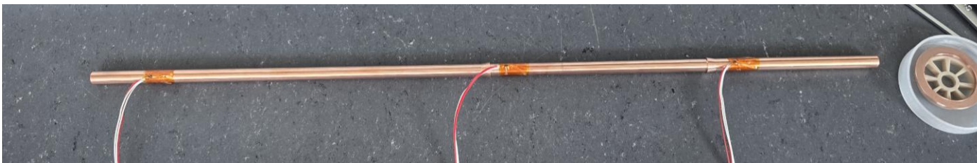
Attaching thermal sensors to inner conductor.
