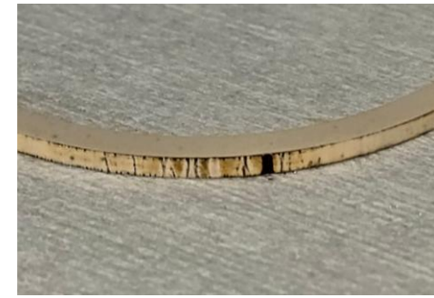
BD damage on outer edge of FE
