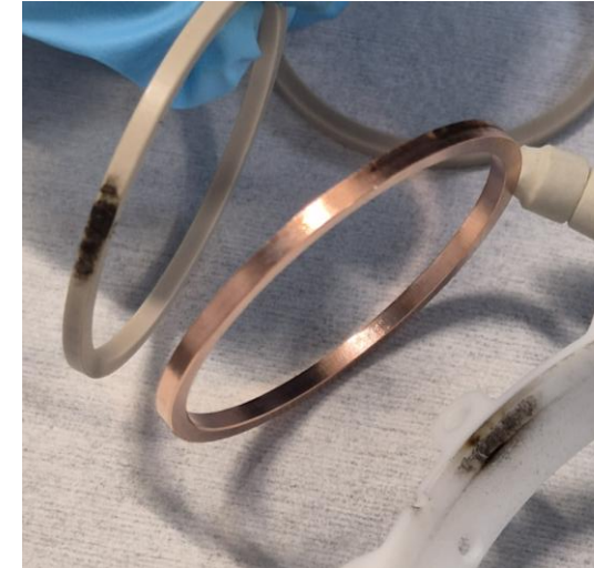
High voltage applied to BE-FRT main body under vacuum, with FE replaced by PEEK.
