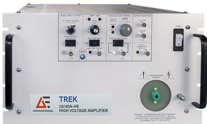
TREK 10/40A-HS high-voltage amplifier
