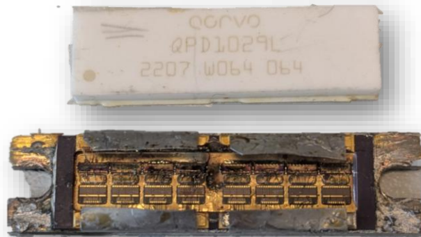
Damaged power amplifier chip on the Qorvo 1 kW SSPA
