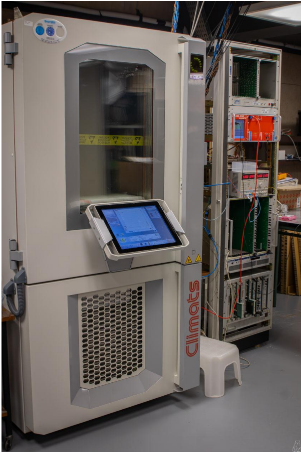
Full e-QC test chain performed in a climate chamber
